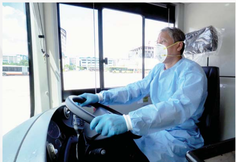
The MAXI features a driver's compartment that is separated by a wall and an emergency door. This is for the safety of all onboard the MAXI.
